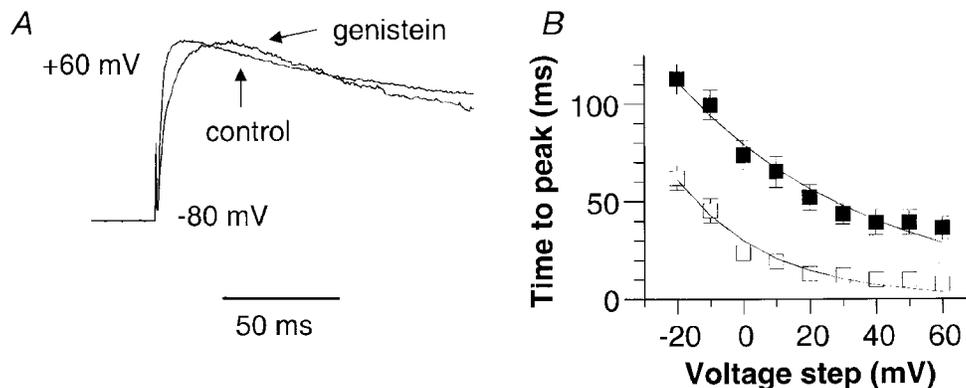
**Figure 4.** Activation kinetics as measured by the time to peak in control and genistein-treated cells
